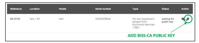
In this case, the broadcaster must extract the BISS-CA public key from the decoder web interface and upload it to <a href="https://www.eurovision.net">www.eurovision.net</a> using the following form:
