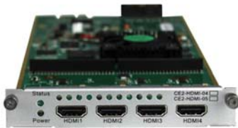
CE2-HDMI-S05: HEVC HDMI Encoder Module (4-CH)
